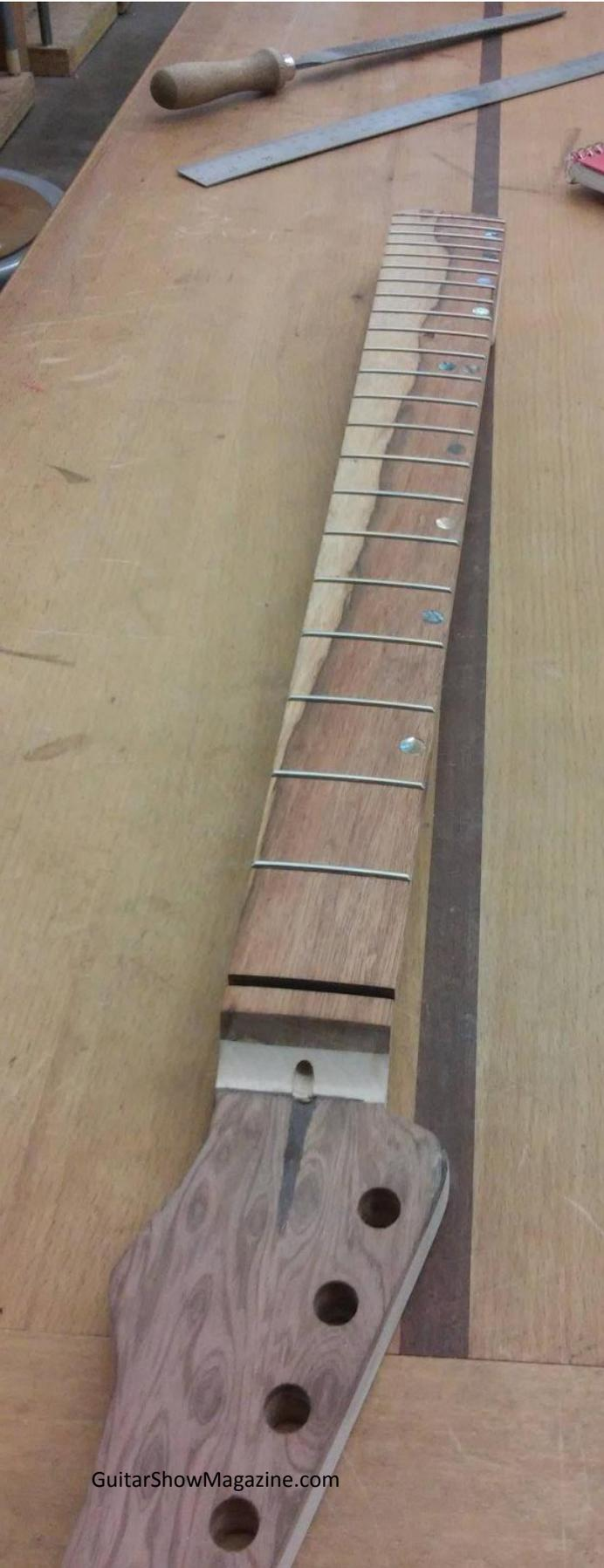
While I did a great job getting the faceplate onto the headstock, I ended up drilling a 2-½ inch long tapered trench in the middle of it for the truss rod access. So now I know to drill the access hole before gluing the faceplate.
